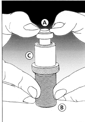
2. With the sealing lips facing away from the tool, slide the “U” cup over the taper on item A.
